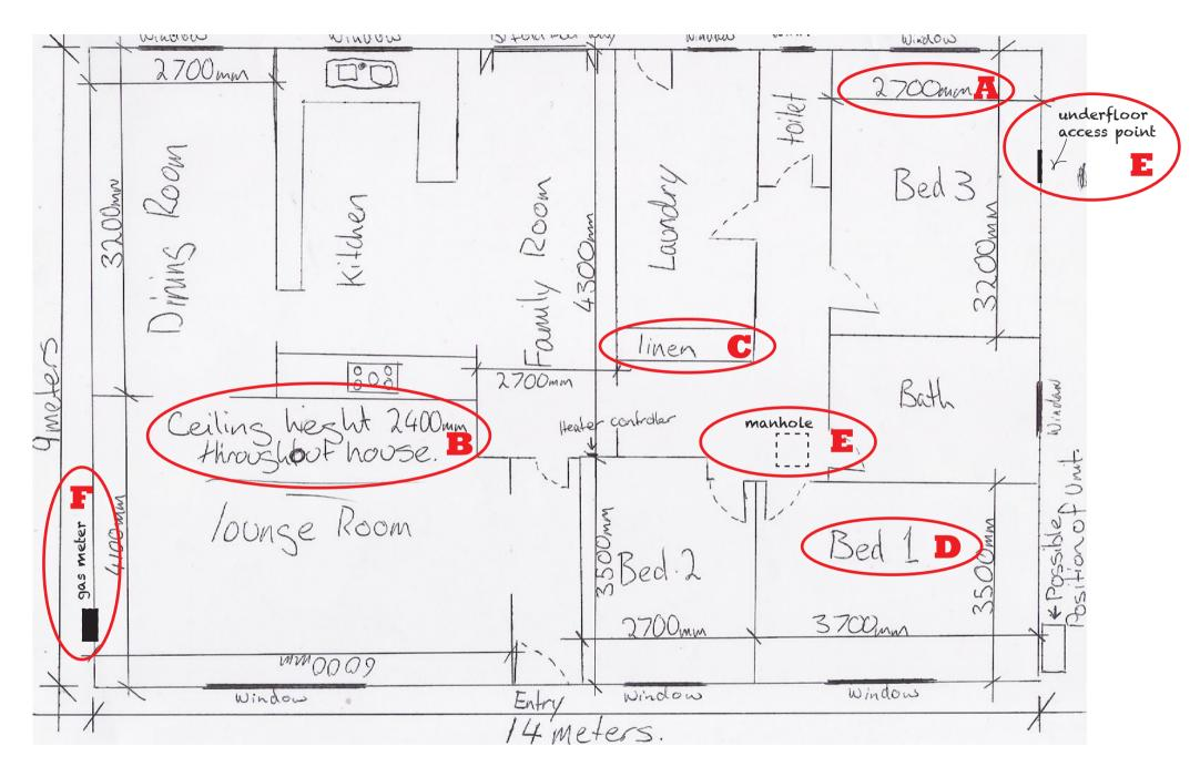
The plan should indicate room dimensions (A), ceiling heights (B), cupboards & wardrobes (C), room uses (D), the manhole and/or underfloor access point (E) and the location of the gas meter/lpg bottles (F) We also need to know if the house is on a slab or has less than 300mm clearance under the house. If there is at least 1m space under the house at the underfloor access point, this should also be noted.
